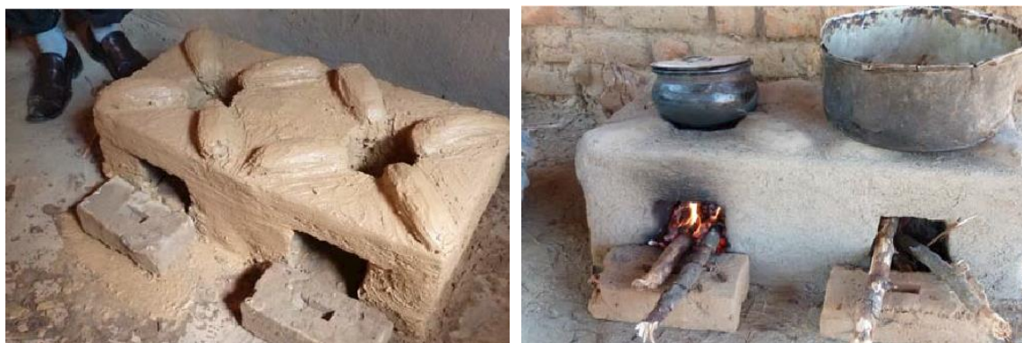
The Changu Changu Moto improved cook stove, recently constructed (left) and in use (right)
